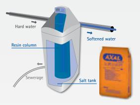
These water softeners are technologically advanced devices whose active component consists of an ion exchange resin for producing soft water. The ion exchange resins replace the "hardness ions" (calcium and magnesium) in the water with sodium ions. Once the resins become saturated with calcium and magnesium ions they lose their effectiveness.
